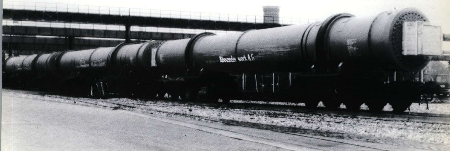
Calciners 2,5 m \varnothing x 23 m long for Alpat Argentine
